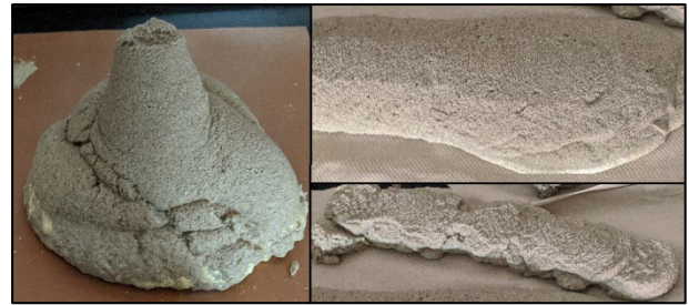
Figure 5 – Test extrusions from the first-generation print head show the variability in the material slump due to changes in extrusion temperature.
