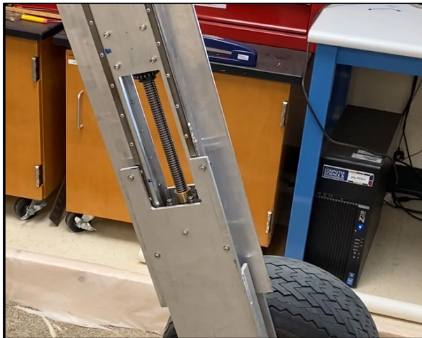
Figure 3. The leg extension mechanism keeps the robot level when traversing obstacles and slopes.
