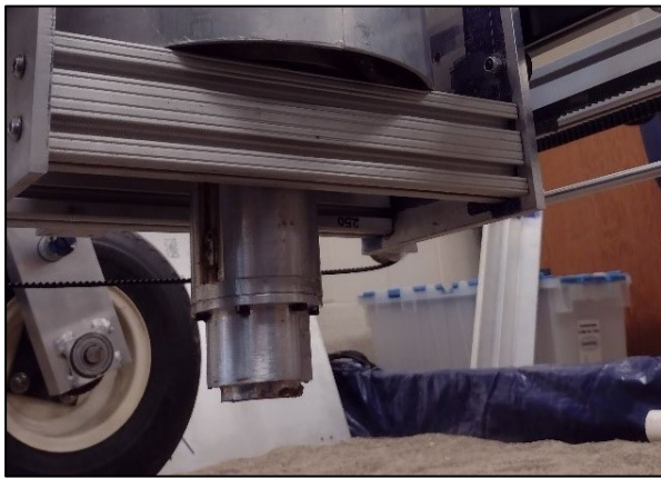
Figure 4. The first-generation print head extrudes a mixture of sulfur and sand.
