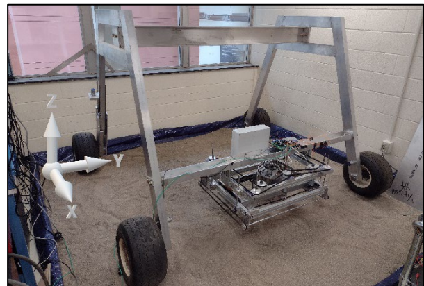
Figure 2. Mud Dauber is a prototype testbed of the mobile gantry architecture.
